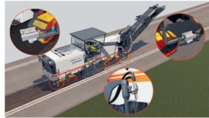
Illustration 8: Large milling machine with multiplex system (example)
